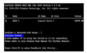
If a critical status error message appears on the FastTrak TX4660 or TX8660 BIOS startup screen for a RAID 1, 5, or 10 logical drive, a physical drive has failed or is not responding. See "Responding to a Critical or Offline Logical Drive" on page 115.
